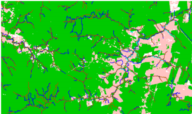
Figure 6. Drainage network for elevation model in orange and drainage network for surface model in blue.
