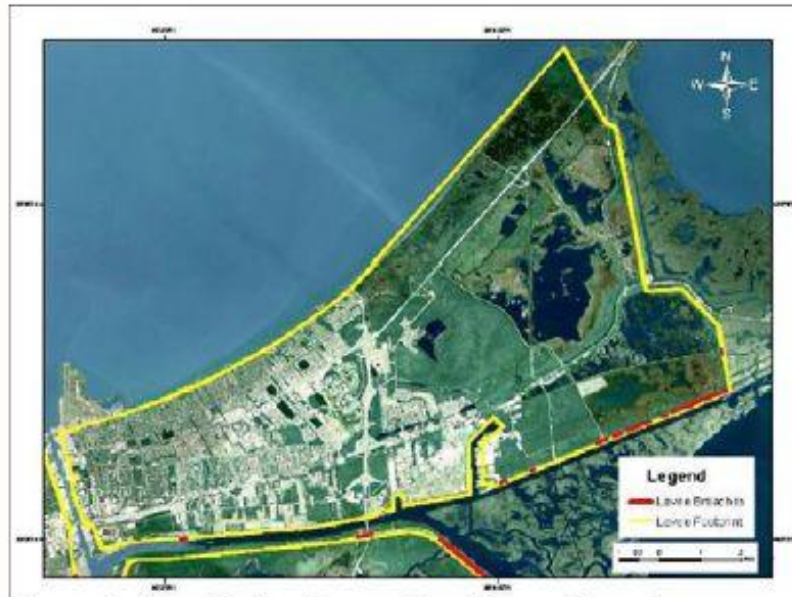
Figure 2. Post-Katrina Levee Conditions Along the Southeast Shore of Lake Pontchartrain.
