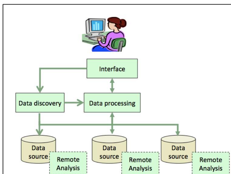
Figure 2 – Proposed architecture for big Earth Observation data processing and analysis.
