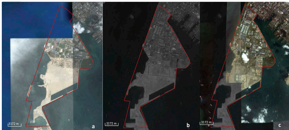
Figure 5. The gradual change in the land cover of the Tuas industrial area (a) 2006, (b) 2008, (c) 2010 (Google Earth, 2015). Also, the activity of dredging through which land is added can be seen over time.
