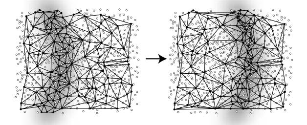
Figure 2: Configuration of sensors and triangulation in response to movement of a front
