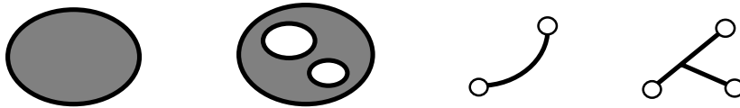
Figure 1: A region with (a) connected and (b) disconnected boundary; and a (c) simple and (d) complex line.
