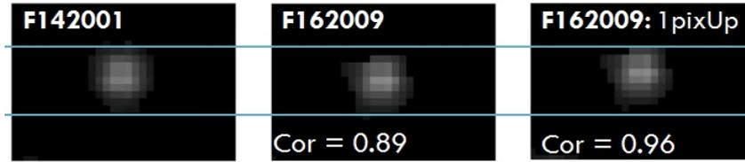
Figure 2.4: Example showing geometric errors in DMSP images. Correlation between F142001 and F162009 images is higher after shifting F162009 one pixel up in vertical direction
