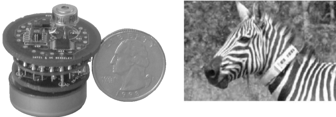
Figure 1.3 - Sensor nodes deployed by the projects Great Duck Island and ZebraNet Project (left and right side, respectively). Left side: MICA-2 (by Intel and University of California- Berkeley). Right side: Sensor necklace.
