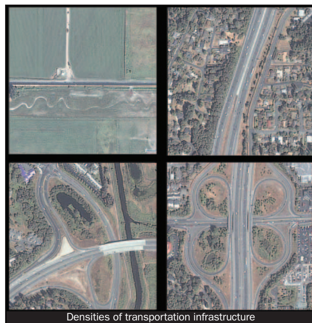
Figure 4. Differing infrastructure densities imply varying degrees of land-cover change and fragmentation in urbanizing areas. Data source: IKONOS 2000.
