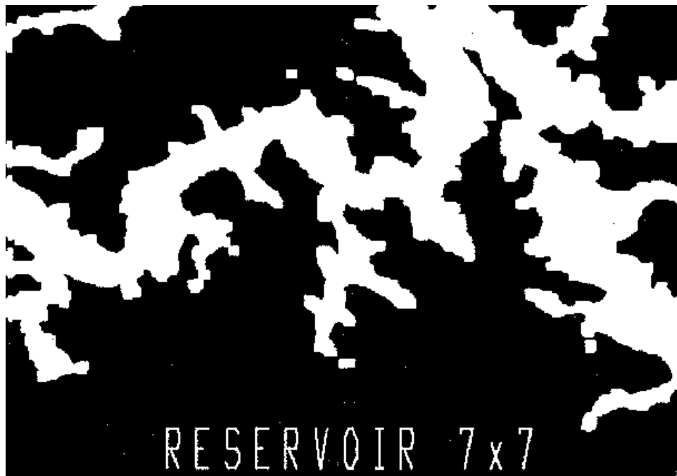
Figure 4 – Reservoir data operated by a 7x7 opening.
