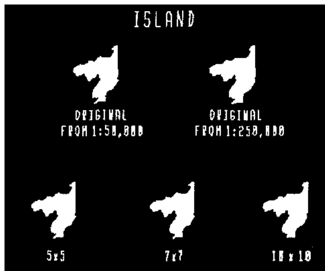
Figure 1 – Ilha Grande, Brazil. The top images were digitized from maps, the bottom ones were automatically generated by MM opening operators.
