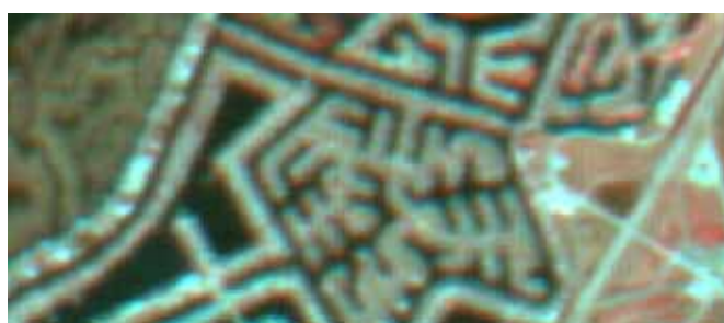
FIGURE 7 – Mismatch between CCD bands 2 and 4
